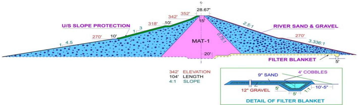
Fig 1. Geometry of Non-Homogeneous Section.
